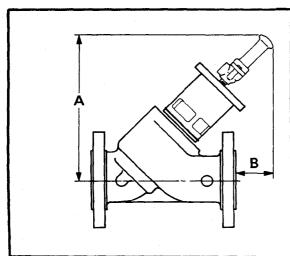
Figure 4-3, Table 4-3 - Clearance Dimensions - Cylinder Removal
